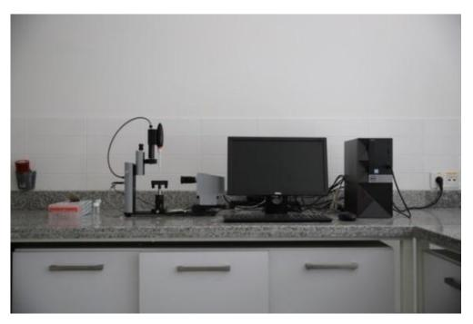
**Intended Use of the Instrument:** Analysis of contact angle, surface tension, and surface free energy of materials
